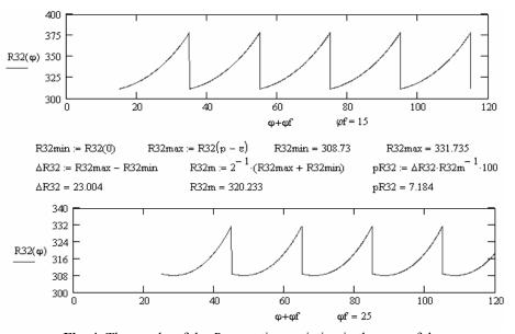
Fig. 4. The graphs of the  $R_{32}$  reaction variation in the case of the gearing line arc angle multiple of the roller teeth step
