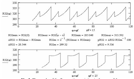
**Fig. 3**. The graphs of the  $R_{32}$  reaction variation in the case of the gearing line arc angle  $\varphi_a = 108^0$  beginning the gearing with the angle  $\varphi_f = 15^0$ , respectively beginning of the gearing with the angle  $\varphi_f = 25^0$
