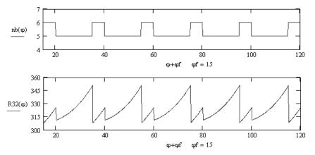
Fig. 2. The variation graph of the  $n_b$  number of roller tooth in gearing and variation graph of the reaction  $R_{32}$  in the case of the some arc of the gearing line
