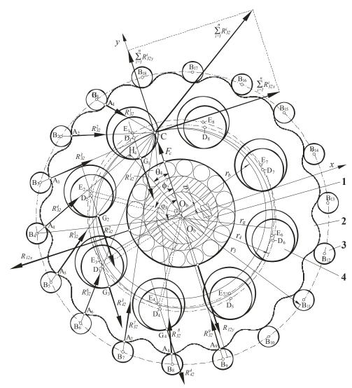
Fig. 1. The reactions who operate on the satellite gear in the case of gearing with  $n_b$  roller teeth
